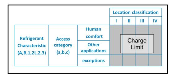
It should be noted that Class 1 and 2 have charge limits, whereas Class 3 systems in general have no charge limitations except for refrigerants in flammability class 3. Machinery room requirements apply at all times. The process can be defined as in the diagram below:
